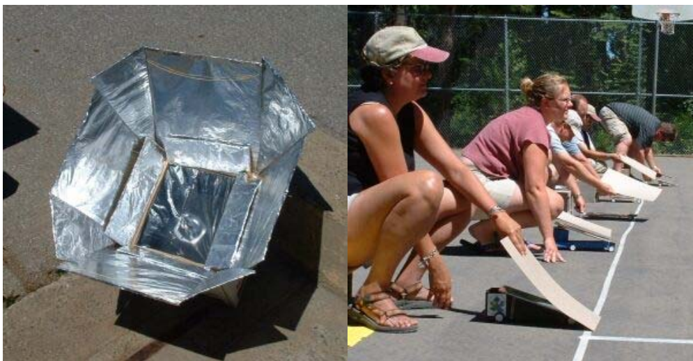
Solar cookers made of cardboard, foil, and plastic window reaches 300F[left]. Teachers ready their solar cars for takeoff. [right]
