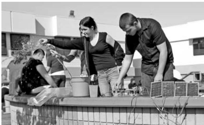
*Students use a Solar Power Monitor to test the pumping performance of four, 3-volt modules wired in series.*
