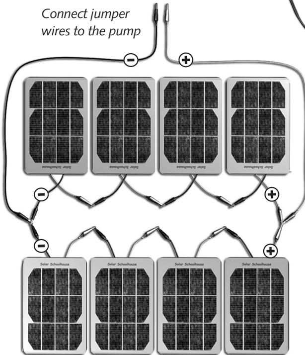
*Attach a second series string in parallel to increase amperage and maintain voltage*
