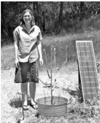
*A moveable tub design with a soldered copper fountain.*
