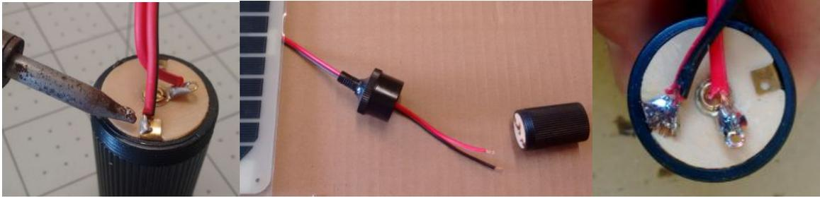
7b. [SOLDER FREE OPTION] Strip ~ ½” of the insulation off of the solar module wires AND the wires attached to the autosocket. Twist the RED (+) wires together and secure with a wire nut. Repeat with the Black (-) wires. Ok to unscrew the cap to see which color wire is connected to the MIDDLE contact. This is Always the Positive (+) contact.
