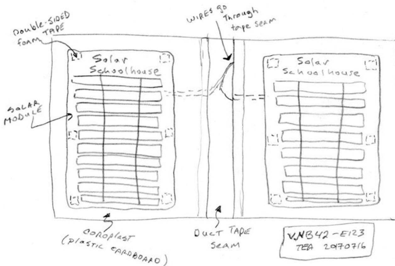
1. Cut two pieces of 4mm thick corrugated plastic (aka coroplast) ~ 7.5" x 9.5". (These dimensions can vary but you should allow minimum 10mm border on all sides around the solar module, with >25-30mm border along the seam). The channels in the coroplast should align with the short (7.5") side, so that one has the option of threading the wires through channels to the seam. Make sure they are roughly the same size. Trim one to match the other, if needed.
