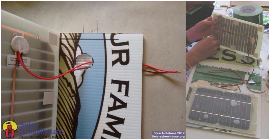
6. Place the Pencil pouch on the back of the notebook. Attach the pouch to the coroplast using zip ties through the two eyelets (pouch) and small holes in the coroplast (using a screwdriver or punch). Then punch a hole through the pouch and coroplast in the corner away from the wires, near the seam. Secure with a zip tie. Cut a small hole in the pouch near the zipper and thread the wires into the pouch.
