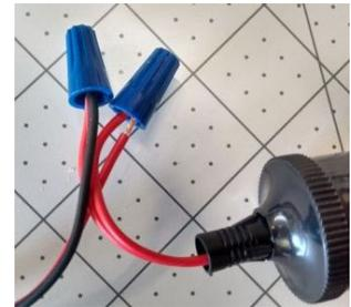
8. Insert the USB Car Charger in the Autosocket. TEST the charger in sunshine and see if the green or red light on the USB car charger lights up. Green (or red) light means it works!!
