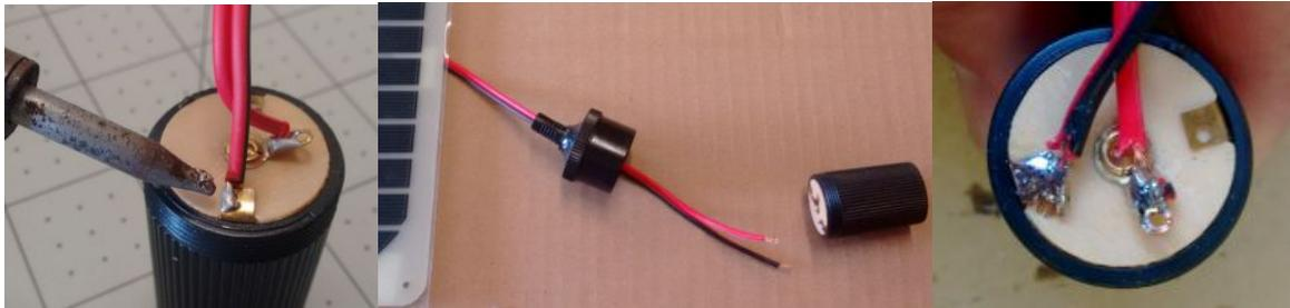
7b. [SOLDER FREE OPTION] Strip ~ ½” of the insulation off of the solar module wires AND the wires attached to the autosocket. Twist the RED (+) wires together and secure with a wire nut. Repeat with the Black (-) wires. Ok to unscrew the cap to see which color wire is connected to the MIDDLE contact. This is Always the Positive (+) contact.
