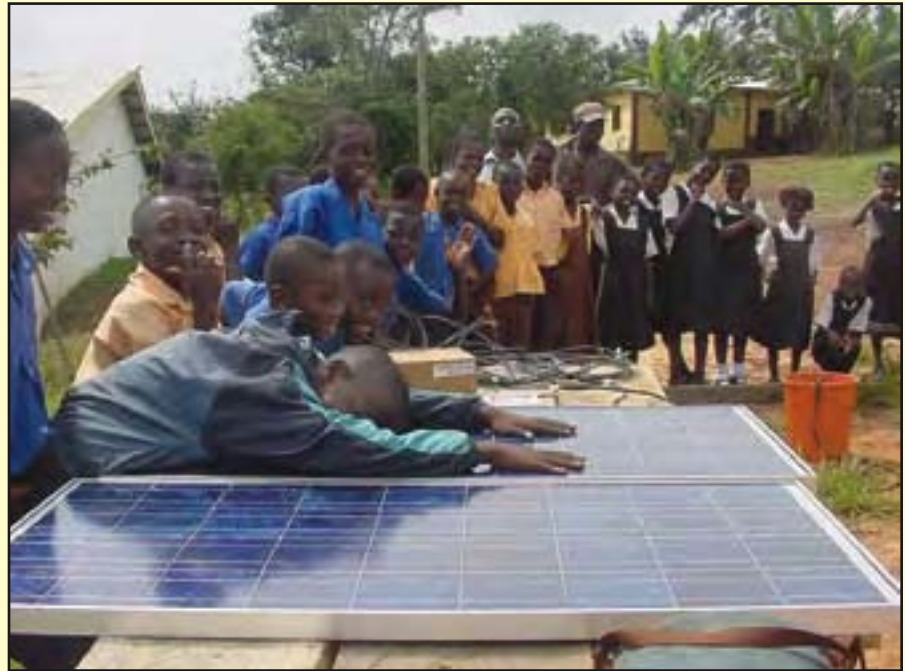
Students learn the fundamentals of solar electricity—the pump stops when a kid shades the PV panels.
