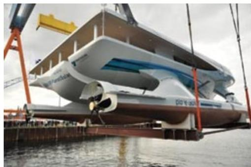
Turanor is fitted with two electric motors - one 20 kW, the other 40 kW - in each float. The solar panels can deliver 94 kW on a bright, sunny day - about five times what the motors need (20 kW) to push the boat at a cruising speed of 7.5 knots, Goulpié says.
