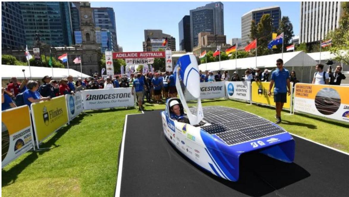
Solar power is a great source of renewable energy, but has always had its limitations. At best, there's only  $1,000 \text{ Watts/m}^2$  available at the Earth's surface on a sunny day, and the limited efficiency of solar panels cuts this down further. It's such a low amount that solar panels on passenger cars have been limited to menial tasks such as battery tending and running low-power ventilation fans.
